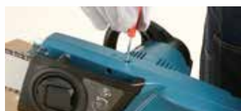
Adjusting the chain lubrication - you can adjust the oil pump feed rate with adjusting screw
